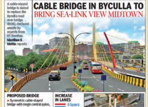
Symmetric cable-stayed bridge with single central pylon, to be positioned in a way to min mise space taken up in market ➤ Long cable span to eliminate need for a large number of foun-dations as exists for current ROB
